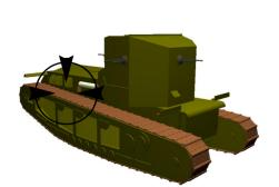
The sides of the Whippet's hull are perhaps the most cluttered parts of the entire vehicle, due to the three vents, exhaust pipe and the complete track unit that is installed on each side. All of these items will be shown in more detail on later pages.
